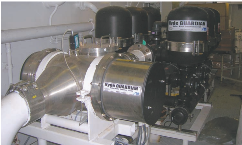
Hyde's modular design, shown aboard the "Mercury", allows great flexibility to install in existing machinery spaces.
